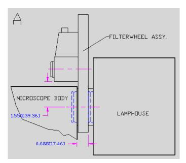
For some microscopes an extender is used with the front adapter to prevent interference of the motor with the microscope body. The length of extenders is reflected in the third column of the table below.
